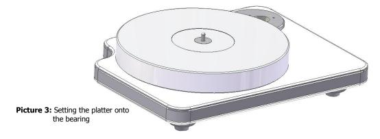
The marks (dots) on the platter and the top of the bearing have been carefully measured. Please make sure they align exactly as shown in the picture.
