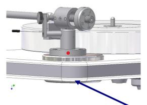
Picture 8: Fixing screw (2) for exact adjustment
