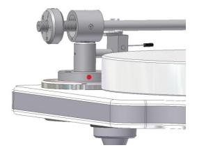
Picture 7: Fixing screw (1) for exact adjustment
