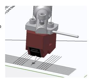
Picture 15: Detail view of cartridge adjustment
