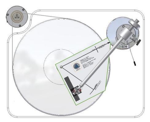
Picture 12: Cartridge alignment gauge
