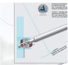
Picture 14: Adjustment of cartridge
