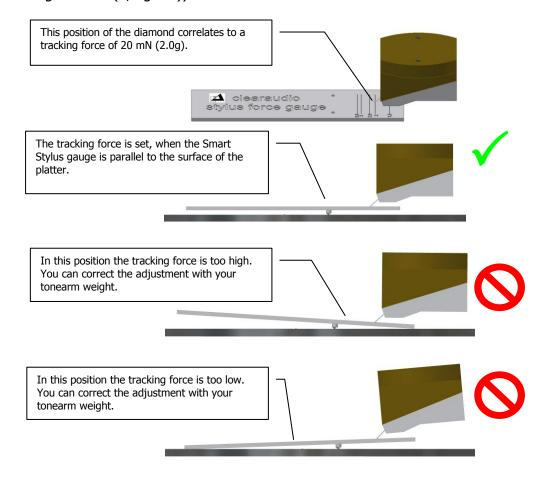
Picture 10: Use of the Smart Stylus gauge
