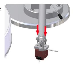
Picture 9: Mounting the cartridge
